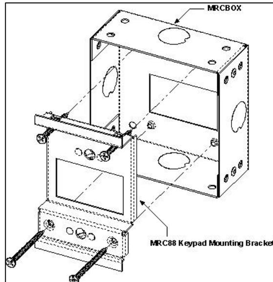
**Figure: Optional Keypad Back-Box for pre-install applications**
